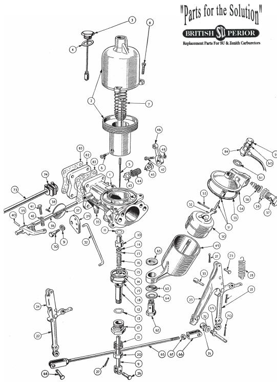
Typical S.U. Carburettor - H Type (Manual Choke)
